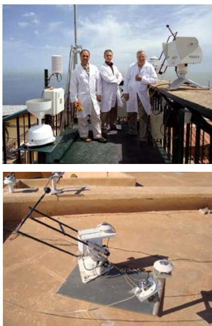
Fig. 2 Sun trackers of Algiers and Ghardaïa stations, CDER
