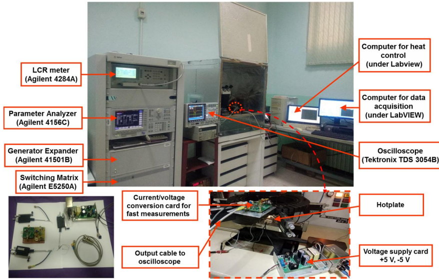
Fig. 26. Experimental Setup _Generation-7 (2018), showing conversion electronic card and instruments used for fast measurements.
