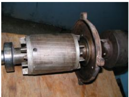
Fig. 5 SCIM with one broken bar
