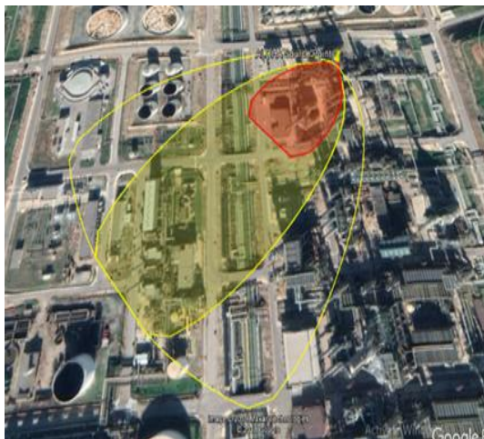
Fig. 6 The threat zone due to explosion in accumulator V 1 (real data)
